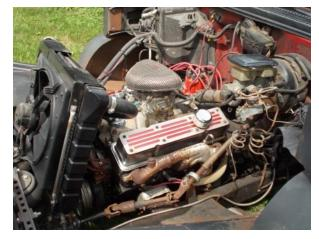
Check out that engine - No word on what it came out of. It's supposedly a Chevy V8 mated to a slushbox trans, Edelbrock air cleaner, carb and intake, plus a dual exhaust with cherry bomb mufflers out the back. Aftermarket valve covers help dress up the...nevermind. Not worth going down that road. This whole thing sits on a "custom built 2x4 hot rod chassis."
